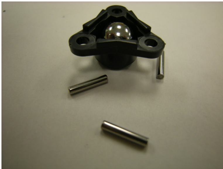
Figure 28: Bearing Rods Before Placement
