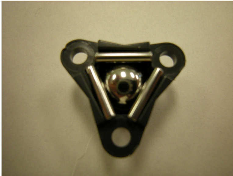
Figure 29: Bearing Rods After Placement
